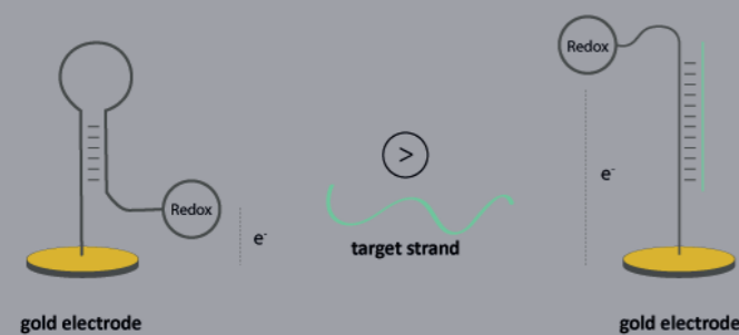
Figure 1: Conformational change of an oligo probe with redox modification before and after hybridisation of a complementary target strand. The change in electrode potential can be finally detected.
